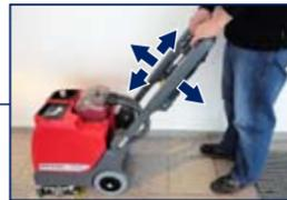
Adjust the handle bar at the correct height (hip level) and tighten the clamp
