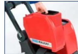
Remove the fresh water and dirty water tank, empty and flush the tanks and the fresh water filter
