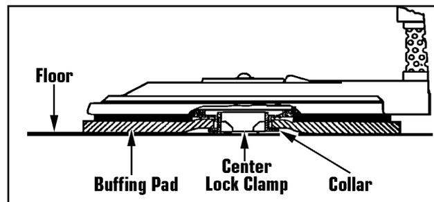
The floor pad packed with this burnisher **MUST BE** attached to pad driver before operating the unit.
