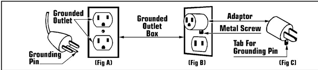
This burnisher is for use on a nominal 120 volt circuit, and has a grounding plug that looks like the plug illustrated in (Fig A). A temporary adaptor that looks like the adaptor illustrated in (Fig B & C) may be used to connect the plug to a 2-pole receptacle outlet as shown in (Fig A) if a properly grounded outlet is not available.
