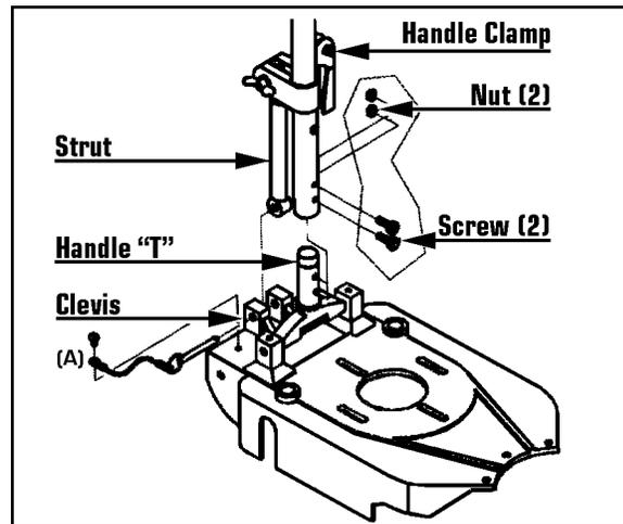
This burnishers is shipped without the handle attached to the chassis. Handle hardware kit (#372811) contains the necessary parts to attach the handle to the burnisher.
