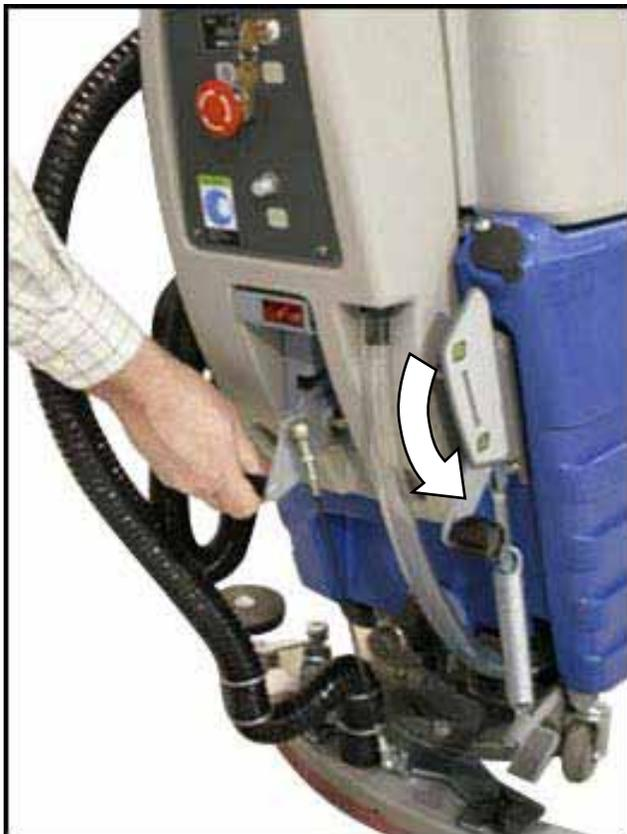
3. Lower scrub head to floor by depressing scrub head lift pedal as shown.
