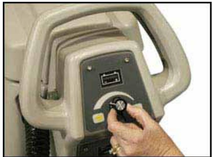
6. Turn the solution flow control dial to desired rate.
