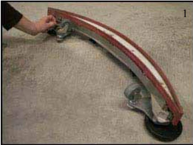
2. To adjust caster height rotate knurled knob for up/down height adjustment.
